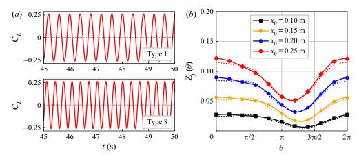
Figure 2. (a) Periodic  $C_L$  oscillation for material types 1 and 8. (b) Comparison of  $Z_y(\theta)$  for different perturbation locations. The solid and dotted lines show the results for material types 1 and 8, respectively.
