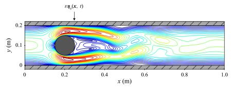
Figure 1. The model used in this study. The elastic structure domain surrounding the fluid domain is marked by the hatched pattern. The cylinder is centred at (x, y) = (0.2 m, 0.1 m).
