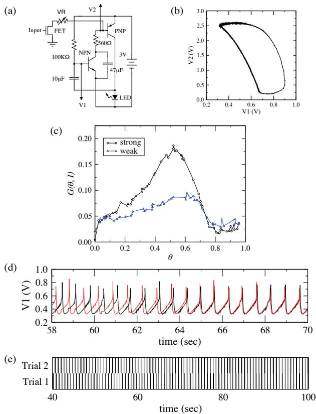
Figure 3: Results of the circuit experiment. (a) circuit diagram, (b) limit cycle, (c) phase maps  $G(\theta)$  obtained using two intensities of the impulses, (d) superposition of two measured temporal sequences of  $V_1$ , and (e) spiking times.
